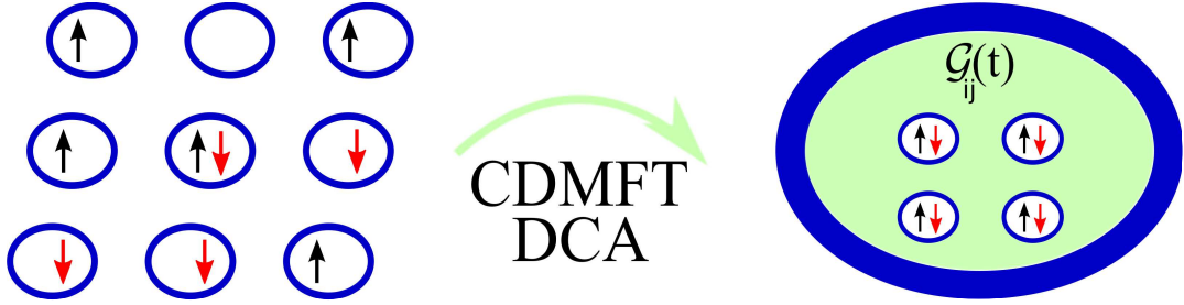
Figure 4.2: Cluster extensions of DMFT: The actual lattice problem is replaced by a cluster of interacting sites, which is embedded into a, self-consistently determined, non-interacting bath, allowing for the inclusion of spatial correlations within the cluster size. Cellular DMFT (CDMFT) and dynamical cluster approximation (DCA) correspond to the two possibilities of considering the cluster in real space (CMDFT) or momentum space (DCA), respectively.
