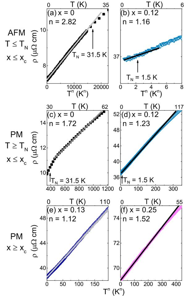
FIG. 2. Resistivity  $\rho(T) = \rho_0 + A_n T^n$  as a function of temperature  $T^n$  for  $\text{Ti}_{1-x}\text{Sc}_x\text{Au}$  for the AFM state (top row) (a),(b)  $x \leq x_c$ ,  $T \leq T_N$ ; and the PM state (middle row) (c),(d)  $x \leq x_c$ ,  $T \geq T_N$ ; (bottom row) (e),(f)  $x \geq x_c$ . (a)–(d) The ordering temperature  $T_N$  is marked by vertical arrows.
