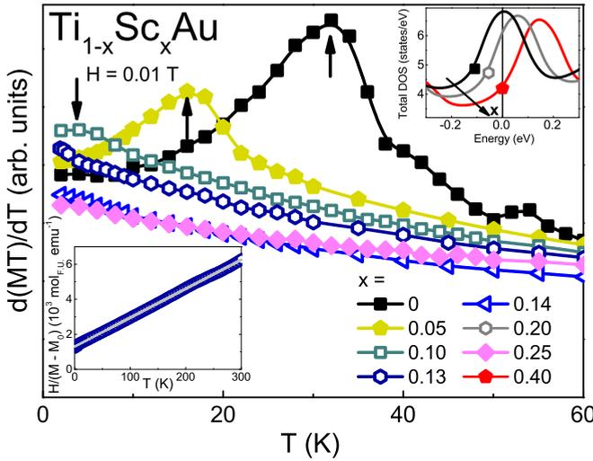
FIG. 1. The Néel temperature  $T_N$  (indicated by arrows) for  $\text{Ti}_{1-x}\text{Sc}_x\text{Au}$ , determined from the peak in  $d(MT)/dT$ . Bottom inset: Inverse susceptibility  $H/(M - M_0)$  (symbols) along with the Curie-Weiss-like fit (line) for  $x = 0.13$  (1 emu = 10 A cm<sup>-2</sup>). Top inset: The density of states calculated for  $x = 0, 0.2$ , and  $0.4$ .
